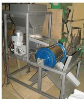
Double Drum Magnetic Separator
