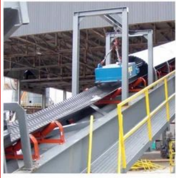
Conveyor Magnetic Separator
