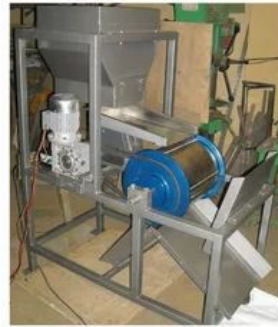
Permanent Magnetic Drum Separator
